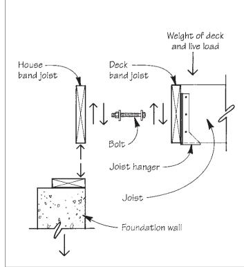
The attachment of a deck band joist to the band joist at the house is a "single shear" connection: two members side by side transferring a vertical load. Bolts (with washers) are the best way to carry this load.
