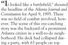
Sixty-three people may seem like a lot, but some easy calculations show that the load on the deck was no more than the building codes say a deck should safely support. The collapsed structure was 25 feet long and extended 12 feet out from the house: 300 square feet of deck.
