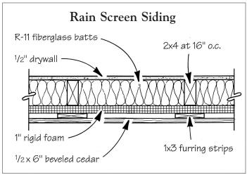
When applying wood siding over rigid-foam insulation, use furring strips to create an air space that buffers moisture cycling.
