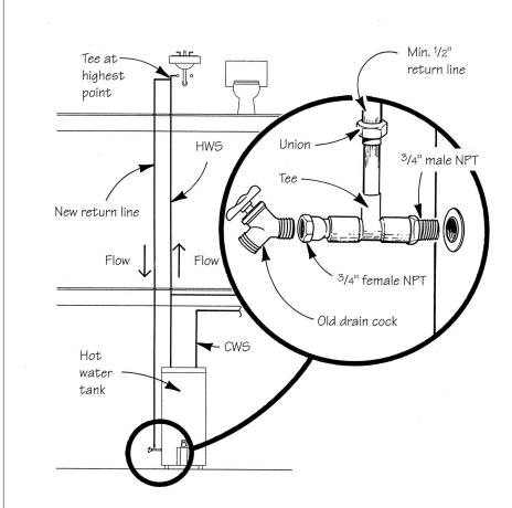
When a sink is located above the hot-water heater, you can provide instant hot water at the sink with a simple passive thermosiphon loop, plumbed with standard fittings.
