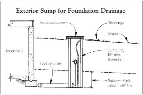
If a sump pump is unavoidable, it should be installed in an outside sump pit with an insulated cover. Make sure the bottom of the pit is below the frostline.
