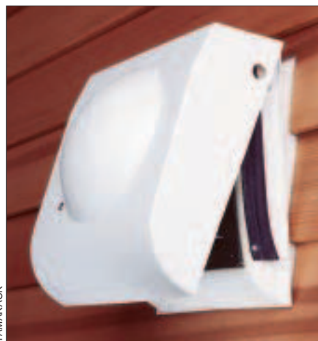
Figure 4. An optional feature of Tamarack's Pre-Ventilator is a motorized insulated door that opens automatically when the fan comes on, then closes tightly to prevent backdrafts when the fan is not running.
