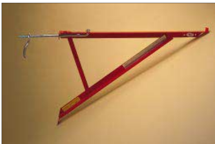
Figure 8. Wall brackets are bolted to wall framing members, and should be spaced no more than 8 feet apart. A railing system or other fall protection is required when the brackets are higher than 10 feet.
