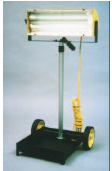
Figure 3. Wide-area fluorescents stay cool and render colors accurately, making them a good choice for finish work. Fostoria's PUL-72F-C Light Cart ($170) casts 5,800 lumens at 72 watts.
