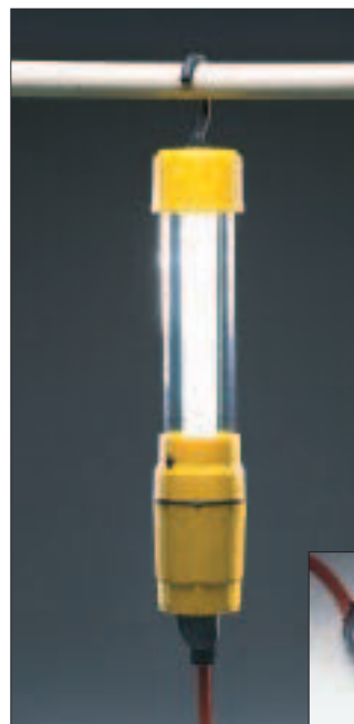
Figure 5. Two new hand lights from Carol have no permanently attached cord of their own, but can be plugged into the female end of an ordinary extension cord. The Plug-It Fluorescent Light (left) uses a cool-to-the-touch 13-watt bulb; the Plug-It Utility Light (below) improves on standard droplights with the addition of a polished reflector to boost output, and a six-sided cage design that helps to hold the light in position against flat surfaces.
