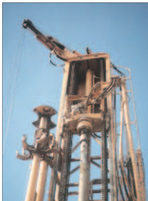
At far left, the truck-mounted drill rig stands in upright position. At near left, the driver, raised to the top of the drilling rig's frame, has just engaged a section of drill rod from the "lazy Susan."
