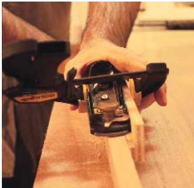
Figure 3. Rather than drag a jointer to the job site, the author uses a low-angle block plane to joint face frame stock. Clamping a guide block on the base of the plane ensures square edges.
