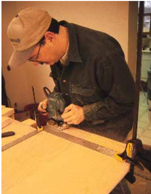
Figure 2. Dadoes cut with a router receive cabinet bottoms (and tops on upper cabinets), while a \frac{1}{4} -inch-deep rabbet accepts the plywood back panel.
