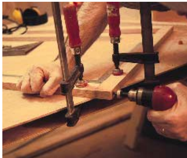
Figure 4. Using a framing square to align the parts, the author glues and screws the face frames together on a flat sheet of plywood.
