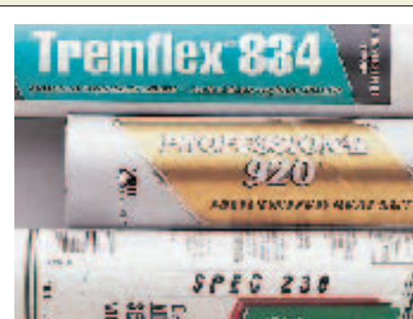
Caulk code: ASTM C-834 is the standard for latex caulks; ASTM C-920 is the spec for sealants for moving joints. TT-S-00230C is a federal standard similar to, and being replaced by, C-920.
