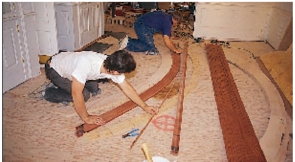
The author and a helper align wood strips in sequence around the bending form.
