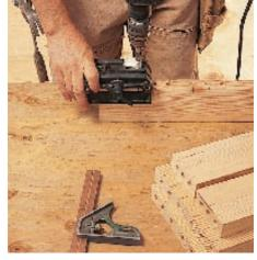
Self-centering doweling jigs ensure that dowel holes are straight and properly aligned. Use a stop collar or a piece of tape to gauge the depth of the dowel holes.
