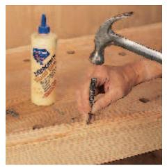
If you're not equipped to mill a profiled glass stop, a glued-and-nailed molding around the inside of the door frame is a low-tech alternative.
