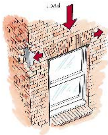
Figure 4. Caution: A loadbearing arch (no steel angle) placed too close to a corner can cause a blowout.
