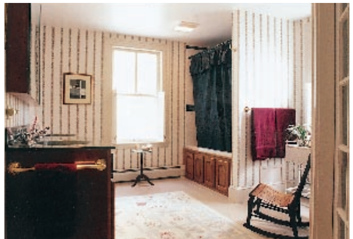
Figure 1. While the room was large enough for a bath (left), the existing window placement and direction of floor joists somewhat limited the choice and placement of the fixtures. Putting the tub in one corner (right) and the toilet on the wall opposite allowed the drain lines to share the same joist bay, limiting demo work and plumbing costs.
