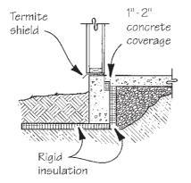
(top sketch) is a bit of a thermal error in that it short-circuits the heat flow from the building, but it should still work against termites. Interior insulation (bottom sketch) may also be an answer, but again there would be some thermal short-circuiting.
