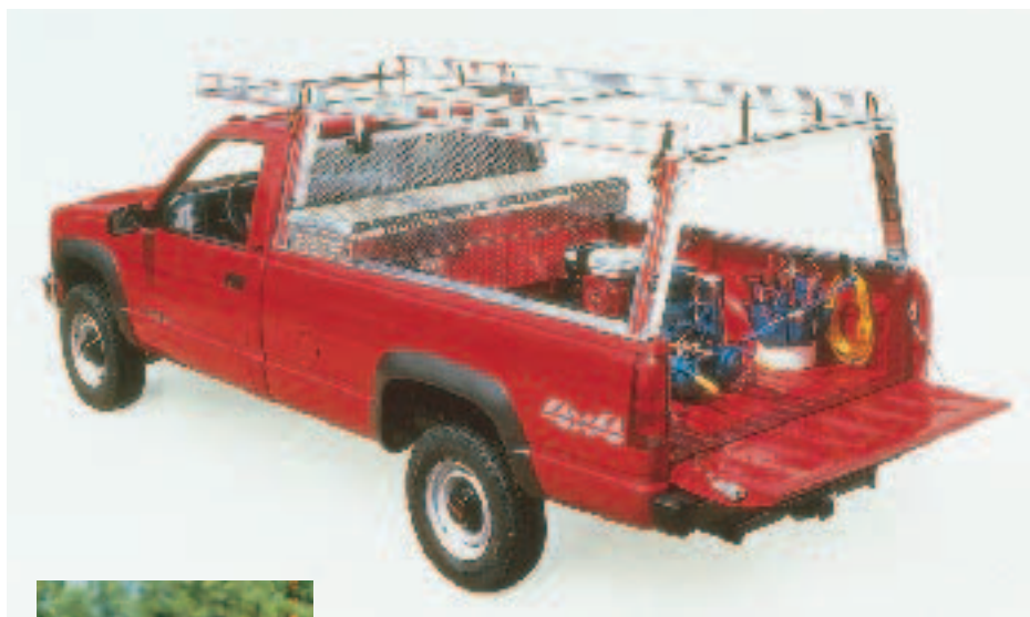
Figure 3. Rustproof aluminum racks are made from slotted and profiled extrusions that allow for flexibility in attaching options like tiedowns and ladder holders. TracRac's uprights (top) can be easily repositioned anywhere along the aluminum extrusions fastened to the sides of the bed, as can the cargo holder in the bed.
