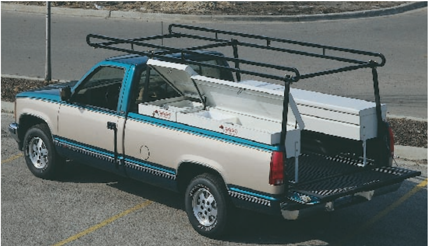
Figure 1. The rear crossmember is the only removable part on a fully welded rack, like this one from McWelco (previous page). Bolt-together racks, like this model from Weather Guard (above), break down into relatively small pieces, so are easy to ship and can adapt to different-size trucks.
