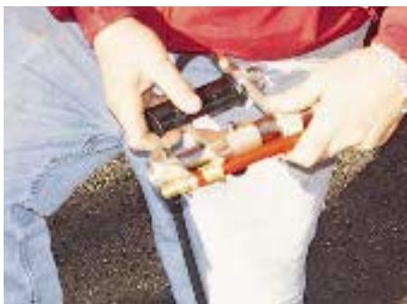
Figure 5. Rehau's joint method uses a foot-operated hydraulic press to force a heavy-duty brass ring over the tube and fitting. The author rarely uses these heavy-duty joints in residential work.
