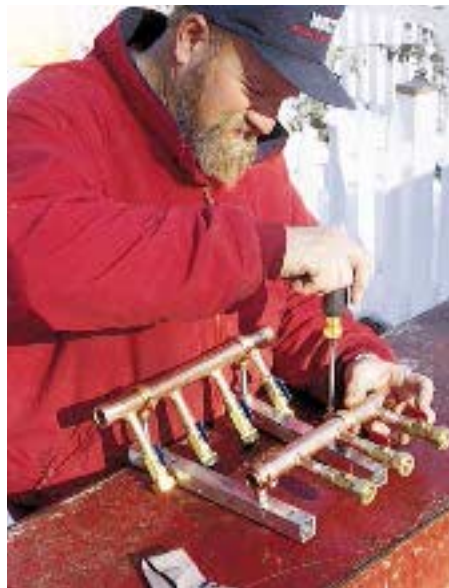
Figure 1. Standard manifolds are available from PEX suppliers (left), but the author prefers to make his own from copper pipe and brass fittings (right).
