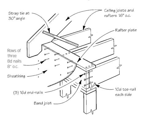
Figure 1. Framing a roof on top of a raised rafter plate allows room for extra insulation above the top plates, but it may weaken the important connection between the ceiling joists and the rafter ends. Using a rated strap tie at every rafter maintains this connection, which helps prevent the roof from spreading. The strap tie also transfers uplift forces from the roof to the ceiling joists.
