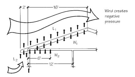
$L_1$  = Roof Lift = 18 ft. x 1.33 sq. ft.\* x 28 psf = 671 lb. per rafter  $L_2$  = Eaves Lift = 2 ft. x 1.33 sq. ft.\* x 28 psf = 75 lb. per rafter Total Lift on Roof = 746 lb. per rafter
