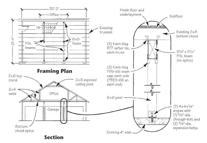
A pair of Parallam PSL beams increased the floor load capacity of these attic trusses from 20 psf to 50 psf. Engineered connections at top and bottom of the posts ensured proper load transfer.
