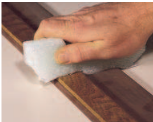
Sponged-back sanding pads are well suited for sanding complicated shapes. The pads work best on finished wood.
