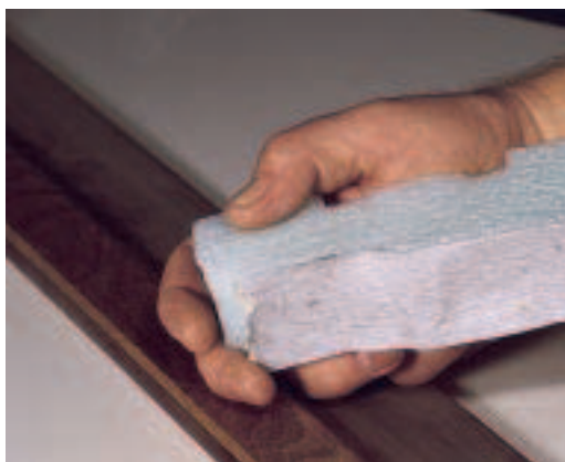
For sanding contours, carve a piece of Styrofoam and use it as a sanding block.
