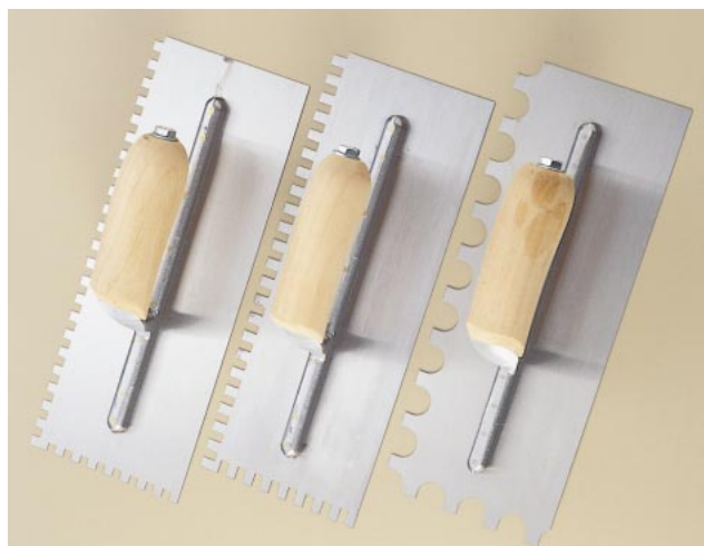
Figure 4. Notched trowels come in many configurations. Shown here, from left, are a 1/4 \times 1/4 -inch notch, for tiles up to 6 inches square, a 1/4 \times 3/8 -inch notch, for tiles up to 12 inches square, and a 3/4 \times 9/16 -inch U-notch, used for irregular handmade tiles.
