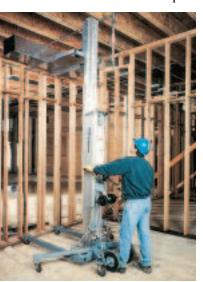
single person to lift up to 650 pounds. The smallest model lifts 6 feet; the largest, 24 feet. Wheels and rollers make loading and unloading a one-man job, and all models fold small enough to fit in the back of a pickup. The 12-foot model weighs just over 200 pounds and retails for around \$1,200.
