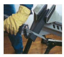
ing the teeth to dull faster. Now, the makers of Lenox-brand blades have introduced the bimetal Demolition Blade, which is thicker and wider than a standard blade, so it cuts straighter and lasts longer. The new blades are available for cutting heavy-gauge metal or nail-embedded wood.
