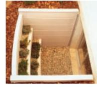
polyethylene walls filled with rigid foam. Panels inside the well provide terraced planter boxes that double as emergency stairs. Installation is quick and easy: Assemble the unit, bolt it to the foundation, then backfill. Wells extend 49 inches from the foundation and are available for 4-foot- and 5-foot-wide windows. Cost is around \$400.
