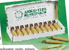
mer in threaded rod or rebar, the polyester resin mixes with the hardener and bonds the stud in the concrete. Unlike expanding fasteners, chemical anchors can be placed near edges, because they don't exert sideways pressure. Sizes are available for  $^3$ /8-inch to 1-inch rod and #3 to #8 rebar. A  $^1$ /2-inch anchor costs around \$3.50.
