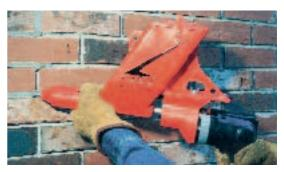
polyurethane hopper holds a <sup>1</sup>/<sub>2</sub>-gallon load of mortar, and an auger pushes the mortar through a steel tip and into the joint; final tooling is done by hand. The interchangeable tips are available in three sizes. The 1764 sells for \$439; model 1864, a lighter version that can be attached to an existing drill, sells for \$259.
