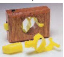
on site, and the result is often damaged doors and door jambs. One easy fix is the Sav-A-Door, a two-piece spring-loaded plastic insert that fits most standard lockset bores. No tools are required for installation just compress the S-shaped handle section, fit it into the lockset bore, and release. A plastic latch piece slides through the edge bore and is adjustable for both 23/8- and 23/4-
