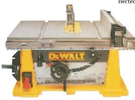
to accommodate rips up to 241/2 inches wide. Rack and pinion gears keep the fence parallel to the blade at all times. The DW744 takes a 10-inch blade, but is comparable in size to other portables. At 64 pounds, it's about 15 pounds heavier
