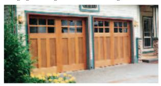
noticed they were really segmented overhead doors. Carriage House Doors are made by applying cedar, fir, or redwood trim to heavy-duty insulated door panels. All doors are made to order, but standard models are available. Delivery takes 6 to 8 weeks, and the manufacturer will quote custom designs in 48 hours. The average installed price is \$2,500 per opening.
