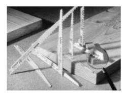
milled blades with similar tooth spacing. Their tips are 8% cobalt, so they resist heat and stay sharp longer than tips made with standard high-speed steel alloys. Fleam Ground blades will cut wood, plastic, and composition materials, but they won't cut nails or metal. Sizes range from 6 to 12 inches long at a cost of \$5 to \$7 each.
