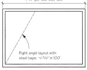
An acceptable tolerance when laying out horizontal dimensions is <sup>1</sup>/4 inch in 100 feet. Variations in right-angle layout should not exceed <sup>3</sup>/4 inch in 100 feet, measured on the diagonal.
