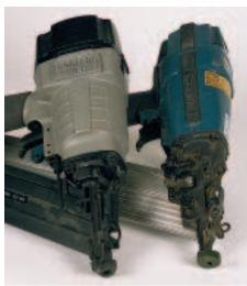
The author found the tip protector on the Makita nailer (right) to be too large, but liked the depth adjuster, which has index points that make it easy to duplicate previous settings. On the Porter Cable nailer (left), the rubber bumper that covers the wire-bale tip is smaller, making it easier to place nails accurately in tight spots. A small, knurled thumb-wheel on the linkage changes the depth of drive.
