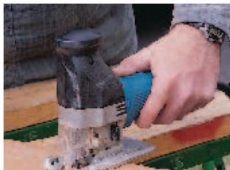
the palm of your hand doesn't cover the switch. Even though I'm right-handed, I like this switch location because some cuts are easier to make left-handed.
