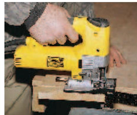
ing it. A quick look at the manual showed that it was really quite simple: Just lift the lever on top of the handle, give it a couple of turns, insert a blade, then turn the lever the other way.
