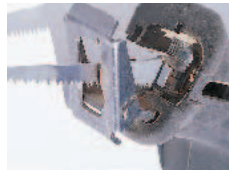
The key-less chuck on Bosch's 1634VS is lever operated and easy to get at, but it won't hold the new extra-thick blades (the key-operated version will).
