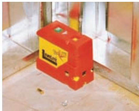
**The pair of perpendicular light beams** projected by the self-leveling LeveLite SLX can be used for laying out square, level, or plumb lines.
