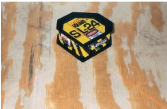
**The SL-24 Laser Square** can project light either as lines, like a rotary laser, or as individual dots, like a point-to-point laser.
