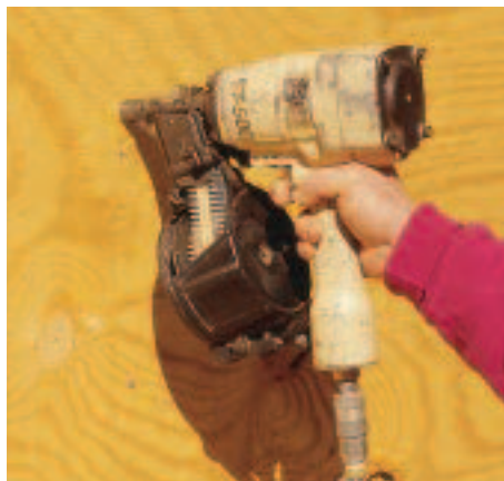
Figure 1. For sheathing, the author uses this ET&F model 500 pneumatic nailer to drive 1 1/4-inch-long nails into 16-gauge metal framing.
