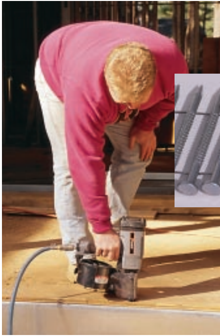
Figure 2. Paslode's model 4250/65 CP-STL drives knurled 1 3 / 4 -inch nails into 14- to 20-gauge steel. In cold weather, Paslode's wire-collated coil (inset) holds up better than a plastic-collated coil, which can break or jam the feed mechanism.
