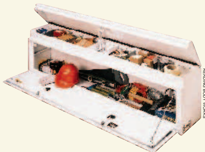
Figure 2. Low side boxes (top) are often used in conjunction with a crossover box. High side boxes leave room for storage underneath, and some have an extra compartment on top (above).
