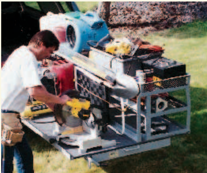
Figure 3. Full-extension sliding beds (left) give the best access to cap-covered pickups. These beds are rated at more than 1,000 pounds fully extended, and can even be used as a work platform. Lighter-duty drawer units are useful in open beds for organizing small tools and parts (right).
