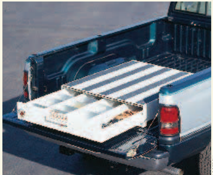
Figure 3. Full-extension sliding beds (left) give the best access to cap-covered pickups. These beds are rated at more than 1,000 pounds fully extended, and can even be used as a work platform. Lighter-duty drawer units are useful in open beds for organizing small tools and parts (right).
