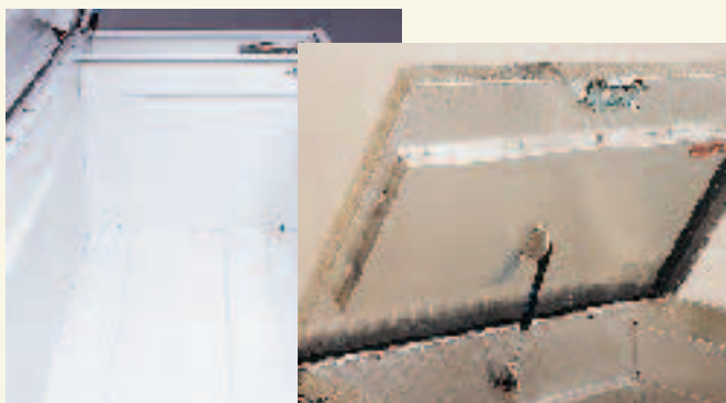
Figure 4. Look for stiffening ribs formed into the bottoms of boxes, which prevent sagging (left). A reinforcing panel tack-welded to the bottom side of the lid stiffens it and prevents it from racking (above).
