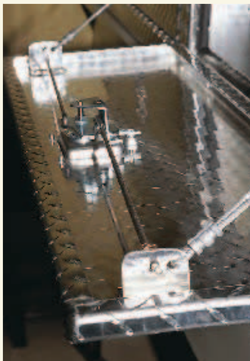
Figure 5. A three-point lock is a good feature on a high side box lid (left). The door closes securely because the latch mechanism engages in the center as well as at the ends. The box above features a two-point lock engaged by a single key at the end. Note also the protective pockets that prevent damage to the piston lid lifters.
