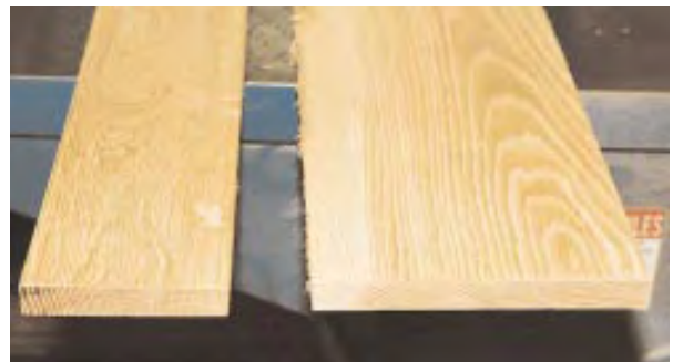
Flooring made from quartersawn lumber (left) will expand and contract much less than flatsawn lumber flooring (right).
