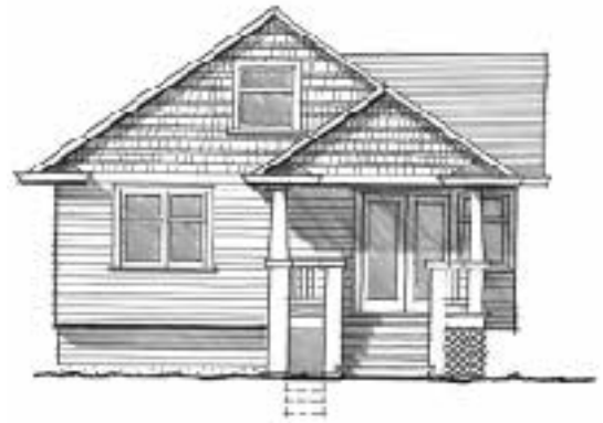
Figure 2. The first proposed solution unified the roofline, but as the clients pointed out, failed to adequately expand the porch while adding upstairs space they never asked for.
