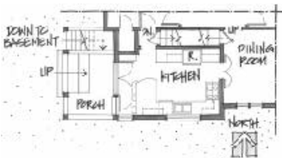
Figure 3. The finished plan not only greatly expanded the porch — one of the clients' chief wishes — but also corrected the eaves and roof massing problems.
