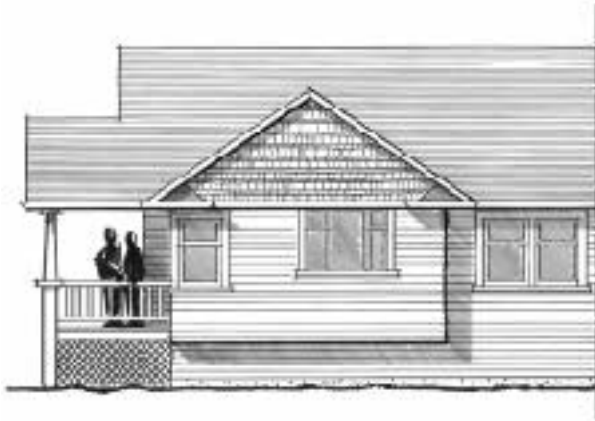
Figure 2. The first proposed solution unified the roofline, but as the clients pointed out, failed to adequately expand the porch while adding upstairs space they never asked for.
