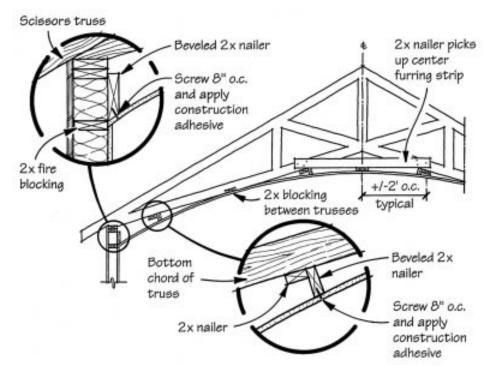
**Figure 2.** It's easiest to frame a barrel vault under a scissors truss. Space nailers 2 feet oncenter, taking care to cut bevels accurately and adding blocking as necessary. To find the location of nailers, use a full-scale layout on the floor if space allows; otherwise, use a scale drawing.
