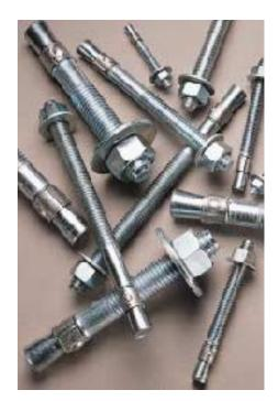
Wedge anchors exhibit the highest holding values among mechanical anchors, but need a strong base material to prevent the concentrated compression forces from pulverizing or cracking the concrete.
