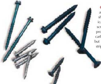
Concrete screws. The tolerance between the screw shank and the pilot hole is critical when using concrete screws. Several manufacturers provide "tolerance matched" carbide drill bits for their screws, but even with these, it's easy to strip the holes if the base material isn't up to specs. In poor
