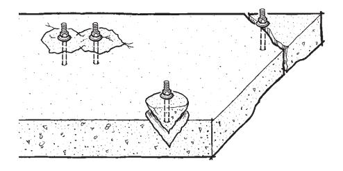
To avoid overstressing the base material, pay strict attention to anchor placement. Manufacturers specify a minimum spacing between anchors to prevent stress areas from overlapping (top left), minimum distance from edges to prevent blowing out the slab (bottom), and a minimum slab thickness to prevent cracking (top right).
