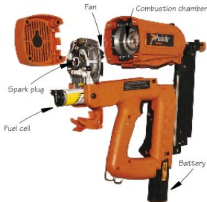
The IM250-II uses a 6-volt ni-cad battery to ignite a spark, and to power a small fan inside the combustion chamber. This fan aids combustion, cools the engine, and blows out the exhaust.
