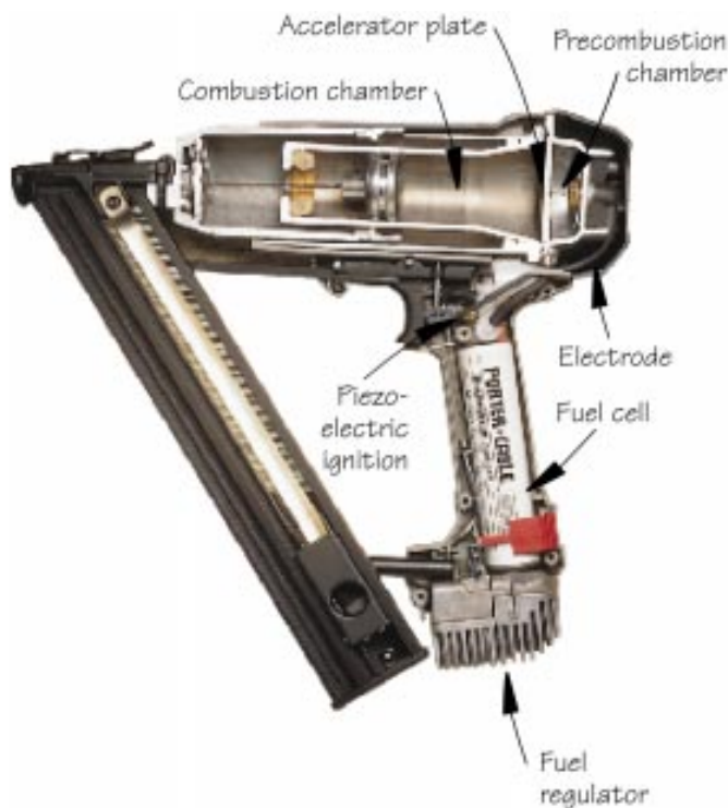
The Bammer engine gets by without a battery using a piezo-electric spark. To fire, the Bammer must be plunged against the nosepiece. This "pump-action" creates pressure differences inside the tool that blend the fuel/air mixture, and push out the exhaust.
