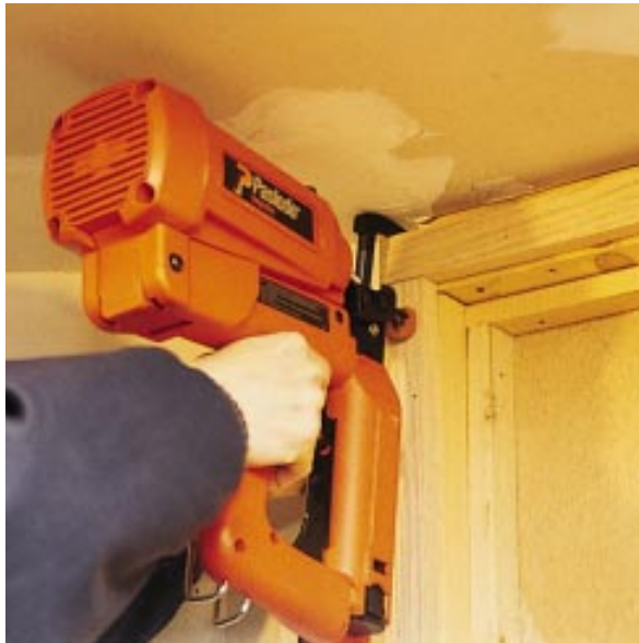
The balance of Paslode's IM250-II makes it comfortable to hold in the vertical position used for the majority of trim jobs.
