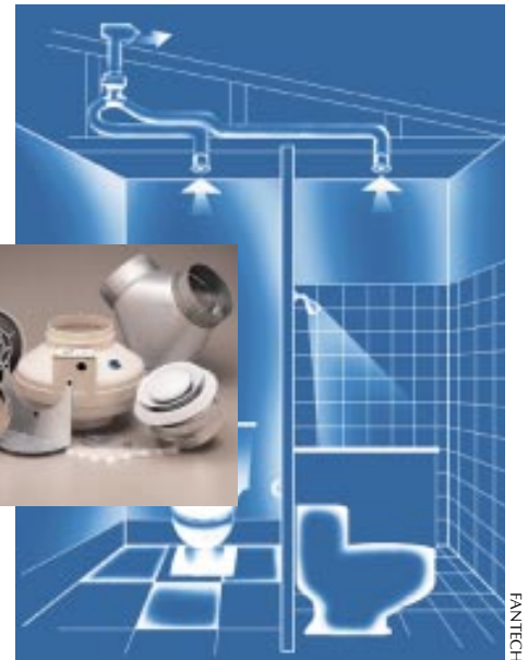
Figure 2. With a single remote in-line fan and a split duct (inset), you can ventilate back-to-back bathrooms or locate exhaust ports directly above more than one fixture.
