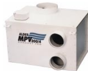
Figure 3. Fans with multiple ports are a convenient way to ventilate up to four rooms simultaneously. A drawback, is that without individual room controls, all areas are exhausted whenever the fan runs.
