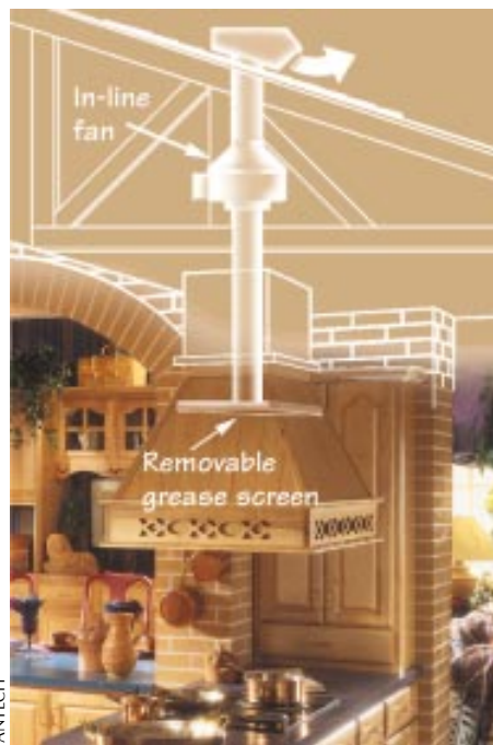
Figure 1. An in-line fan located in the attic is quiet when running at high speed. With a variable-speed switch, the fan can be run at low speed during meals to keep food odors from permeating the rest of the house.
