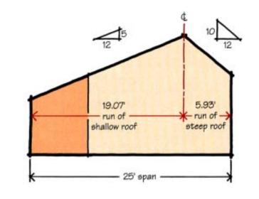
Using the "equalized" span, follow the four-step process from Case 1 to find the run of the steep roof:
