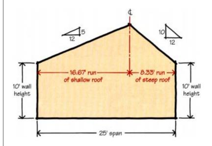
**Step 1.** Add the rise of the two different roof slopes: 5 + 10 = 15.
