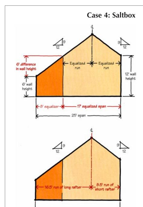
A Saltbox is a standard gable roof set on walls of unequal height. To lay out the rafters, first follow the three-step process in Case 2 to "equalize" the span.
