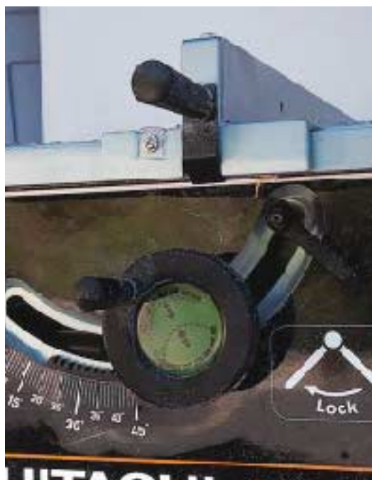
Figure 3. By pushing the height-adjustment wheel toward the housing, the Hitachi saw allows you to micro-tune the bevel setting.
