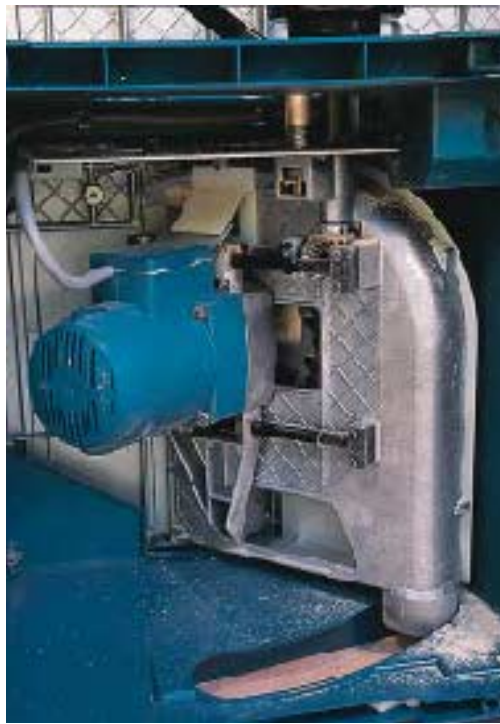
Figure 4. Like the other new portables, the latest Makita table saws have an enclosed blade housing inside the cabinet for improved dust collection.
