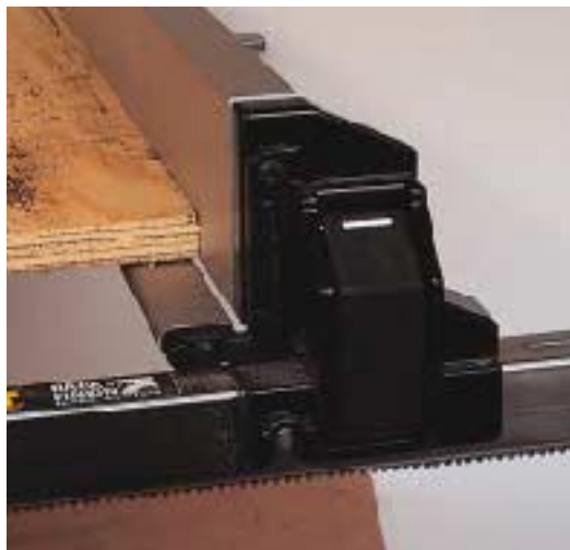
Figure 2. The rack-and-pinion action of the DeWalt fence is precise. The author found it reliable enough that he no longer needed to pull out a tape when repositioning the fence.
