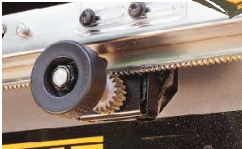
Figure 1. The two extendible rails on the DeWalt table saw ride on rack and pinion gears. These gears provide smooth action and ensure parallel positioning when adjusting the width of a rip.
