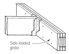
**Sideloaded beams must be carefully nailed together,** to ensure that all the beam members share the load.
