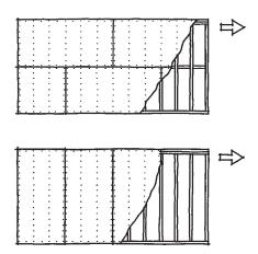
When all the panel edges are supported by solid framing, 1/2-inch plywood sheathing is stronger against racking forces when installed horizontally (top sketch). If there's no blocking at the 4-foot mark, the sheathing is stronger installed vertically, as long as all edges are supported (bottom sketch).
