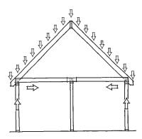
Collar ties are usually not needed in conventional gable roof attics, as long as the floor/ceiling joists are properly connected to handle the tension forces created by the outward thrust of the roof.
