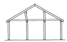
**Purlins and struts reduce rafter spans** just as bearing walls do. The struts, or a kneewall, should be installed as close to vertical as possible, and must be properly supported below.
