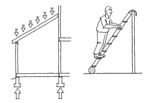
Collar ties are not necessary in a cathedral shed roof, since there's no outward thrust to restrain. The situation is analagous to a ladder leaning against a wall, and attached at the top. Even if it's on wheels, the ladder can't move away from the wall.
