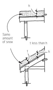
When adding up the weight of snow of a sloping roof, use the horizontal run of the roof, since the same amount of snow would accumulate on a perfectly flat roof. The code also allows you to apply a slope reduction factor, to account for snow blowing or sliding off a sloping surface.
