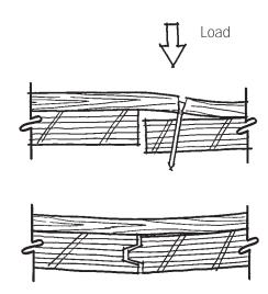
Unsupported joints in square-edged plywood floor sheathing cause squeaks when someone steps on them. T&G plywood sheathing prevents squeaks and makes the floor feel stiffer, though it doesn't actually increase the design strength of the floor system.
