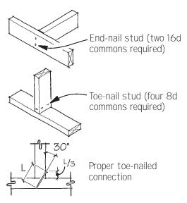
When nailing a stud to a plate, a toe-nailed connection is typically stronger against lateral forces than an end-nailed connection.
