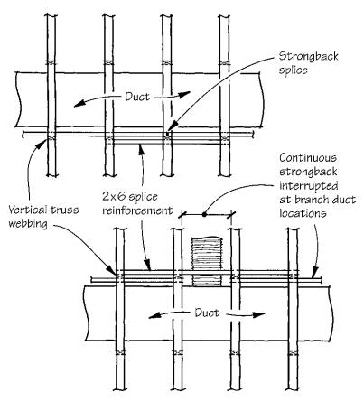
The strongback for a truss floor should be fastened to one of the vertical webs at the hvac opening provided at centerspan. Reinforce splices with a 4-foot-long member on the opposite side of the vertical web (middle). If you need to make room for a branch duct, you can leave a gap in the strongback and reinforce it with a 6-foot piece that catches four trusses (bottom).
