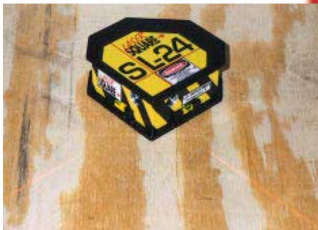
Figure 3. Square lines. More of a layout tool than a long-distance leveling tool, the Laser Square gives you visible lines at a right angle. For some layout jobs, such as laying out floor tile or leveling a countertop, it's more useful to have actual lines to sight along than a single reference dot.
