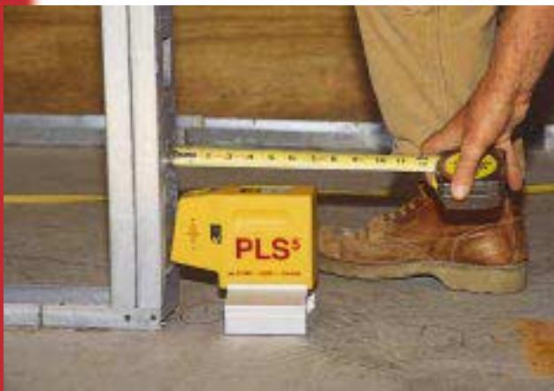
Figure 2. Plumb, level, square. Accurate to \frac{1}{8} inch over 100 feet, the self-leveling PLS5 is one of the most exact instruments among the new breed of lasers. It has two plumb beams (one up and one down) and three level beams (at 90 degrees to each other), so you can accurately mark both ends of every layout line.
