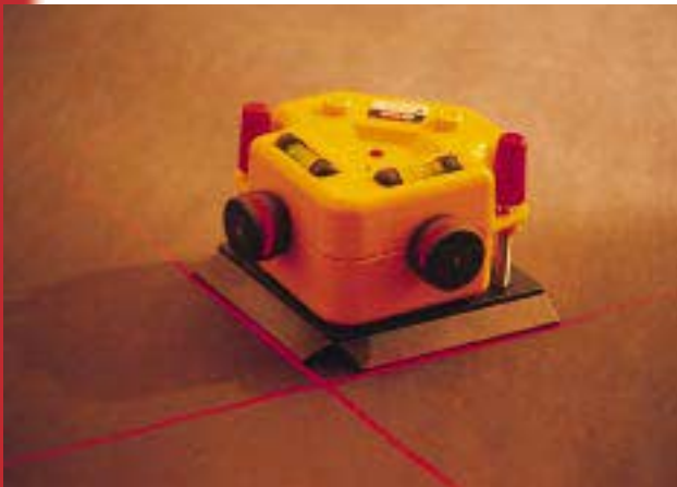
Figure 5. Rotary square. The Momentum DP 90 features two rotating diodes positioned at right angles. These project visible right-angle lines on the floor, as shown, as well as on the ceiling and walls.
