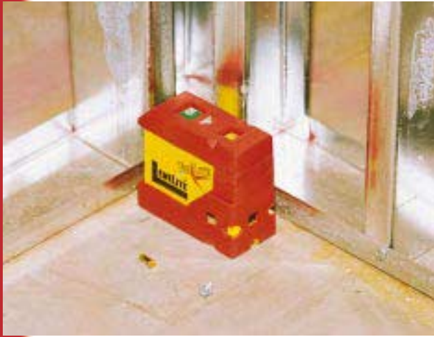
Figure 1. Square dots. Though not much bigger than a tape measure, and nearly as durable, the Tri-Lite has won fans in the commercial interiors market for quickly plumbing steel partitions. The unit is self-leveling and accurate for distances under 50 feet.
