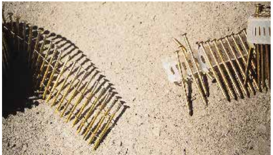
Figure 1. Wire-collated nail coils (left) can stand up to getting dropped or carried in nail bags. Plastic-sheet collated coils (right) tend to fall apart with even the slightest mishandling.
