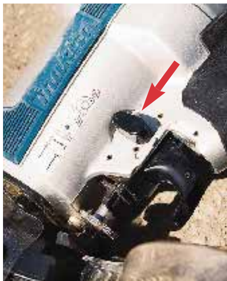
Figure 3. Makita has added a safety-select switch (see arrow) to the trigger. One position allows you to bounce-fire; the other limits the gun to sequential-trip firing.
