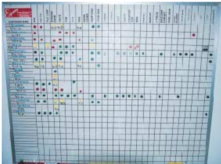
Figure 2. The author's job board helps keep four-day bath jobs on schedule. Red dots mean a part needs to be ordered. Yellow dots indicate the date the part should arrive. Green dots give the go-ahead — the part is in and has been inspected.
