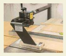
instead, it must be positioned vertically and horizontally before making a cut. The anti-kickback device can be retracted and locked away from the work to avoid marring, and the entire saw guard rotates out of the way when blades are changed or adjusted. Brett-Guards are available for 10- to 16-inch saws at prices ranging from \$278 to \$560 depending on blade size and mounting options.
