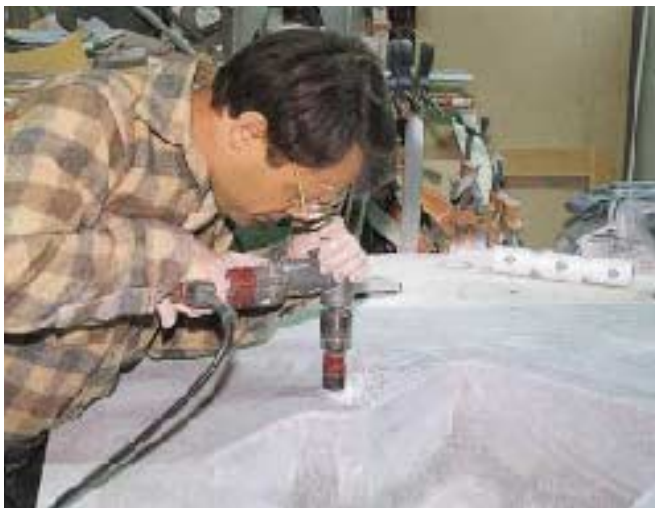
Figure 5. Deep-throat vise-grip clamps hold the undermount sink in place while the adhesive sets (far left). After the top is routed flush with the sink edge (middle), the author bores holes for the faucet with a carbide-tipped hole-cutter (left).
