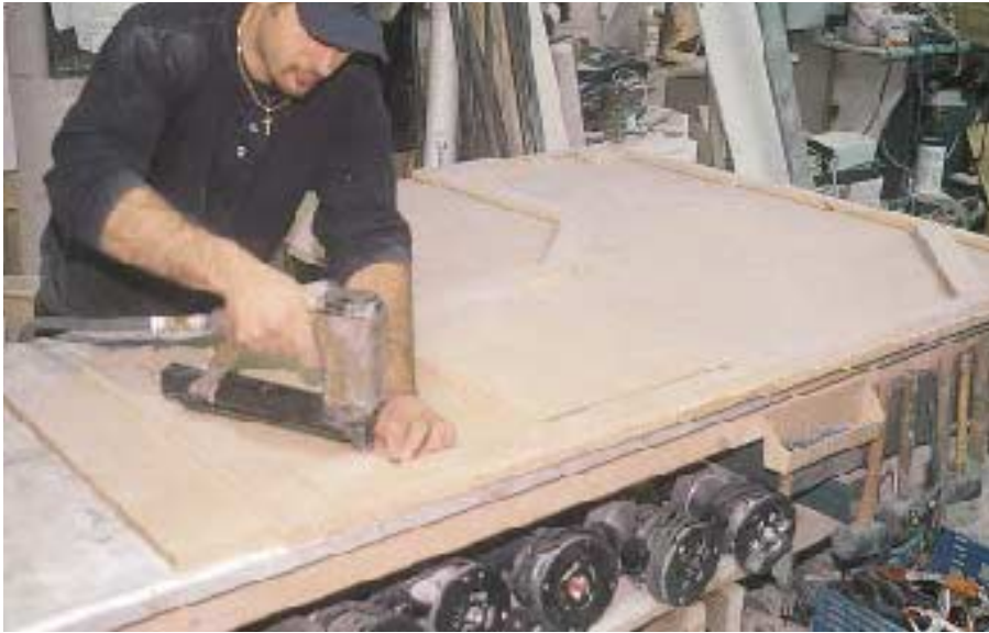
Figure 1. Working to layout lines, the fabricator glues and staples edge buildup strips in place (above). The top is then flipped over and routed flush to the buildup strips. The final step in preparing the substrate is to cut an expansion kerf \frac{3}{4} inch in from the edges, per the manufacturer's instructions (right).
