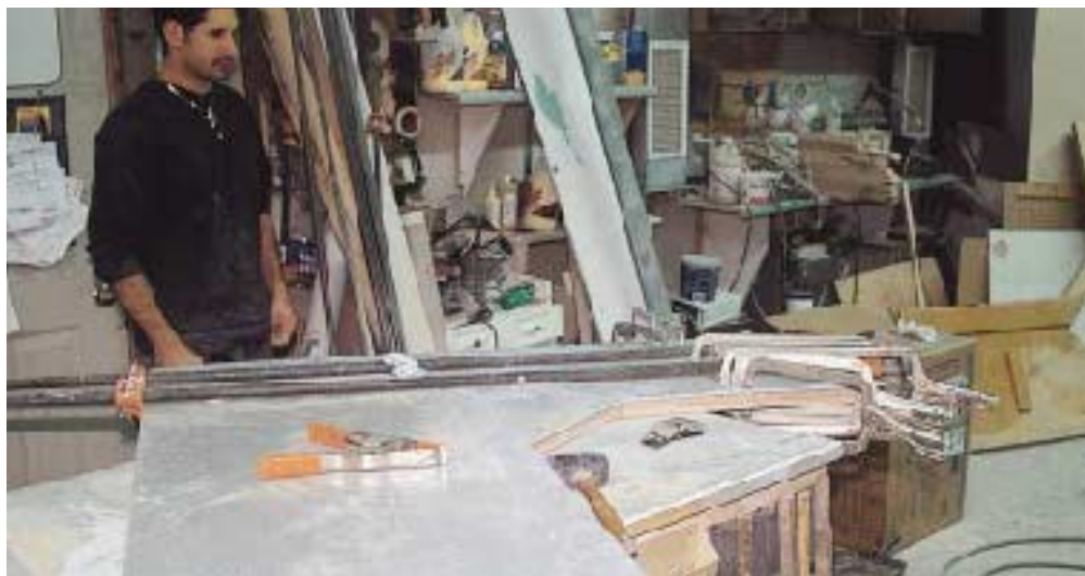
Figure 3. Gluing up Swanstone is much like gluing up laminate: Contact cement is spread on mating surfaces, and dowels are used as spacers while the solid surfacing is positioned (far left). At seams, acrylic adhesive is applied to mating edges and the Swanstone insert (middle). The author uses pipe clamps to secure the joint while the adhesive sets (left).
