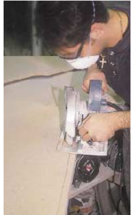
Figure 1. Working to layout lines, the fabricator glues and staples edge buildup strips in place (above). The top is then flipped over and routed flush to the buildup strips. The final step in preparing the substrate is to cut an expansion kerf \frac{3}{4} inch in from the edges, per the manufacturer's instructions (right).
