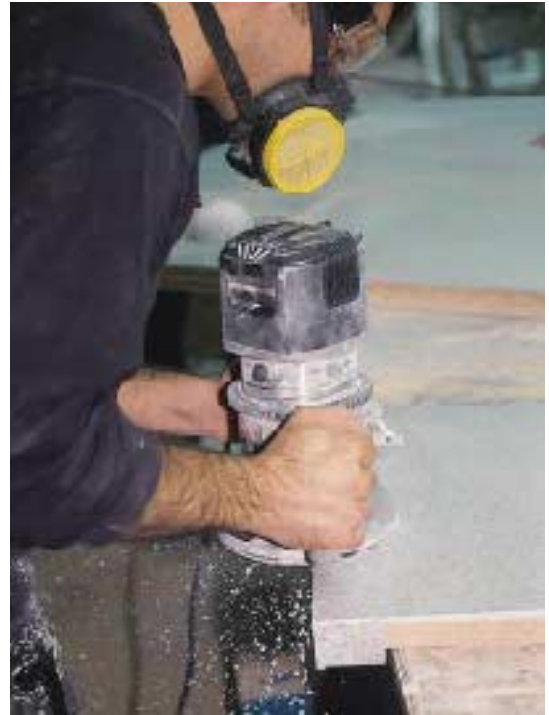
Figure 4. With the top flipped upside down, the edge banding is attached with acrylic adhesive and spring clamps (above). The edging fits tight against the bottom of the overhanging top surface. After the glue sets, the counter is flipped over and the top is routed flush with the edging.
