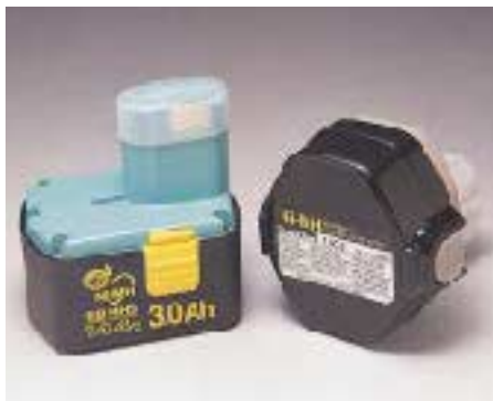
Figure 1. Nickel metal hydride (NiMH) batteries like the 2.2Ah from Makita and 3Ah prototype from Hitachi increase runtimes for each charge. However, they are more expensive than more common NiCad batteries and cannot be charged as many times before wearing out. With the added runtime, though, manufacturers are claiming that NiMH total runtime over the life of the battery is still greater than with NiCads.
