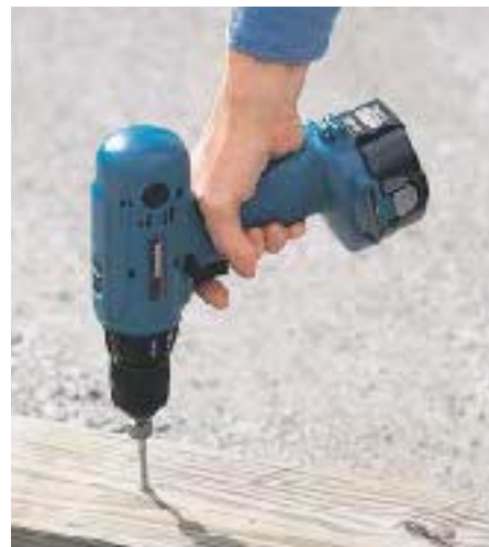
Figure 2. The DeWalt and the Makita drills had the best overall maximum power — evident from driving lag bolts into a pressure-treated pine 6x6.
