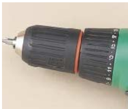
Figure 4. Chucks on the Bosch, Panasonic, and Hitachi (shown here) are easy to grasp and adjust with one hand.
