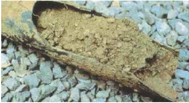
Figure 6. Regardless of the type of pipe used or its shape, unfiltered drain tile can easily be plugged with silt and clay (left). Water-seeking roots from trees growing too near the foundation can also completely clog perimeter drains (right).
