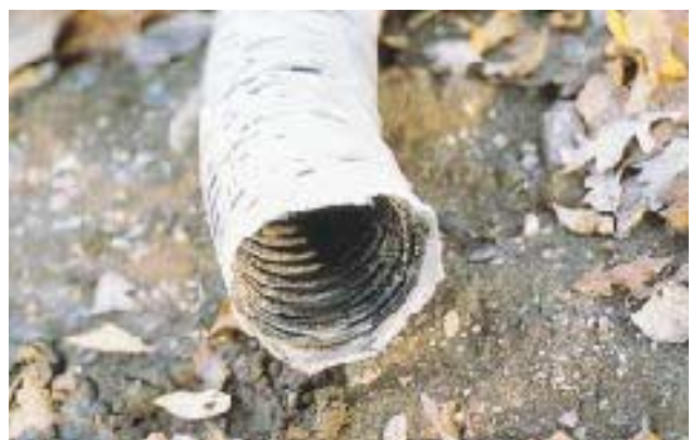
Figure 4. Without a filter to keep silt from contaminating the surrounding stone, drain tile can be rendered useless within just a few seasons (left). Pipe that is pre-wrapped or "socked" with filter material will prevent drain tile from becoming plugged (above).
