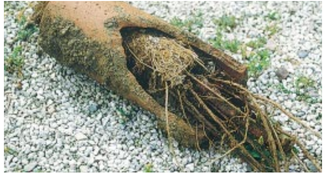
Figure 6. Regardless of the type of pipe used or its shape, unfiltered drain tile can easily be plugged with silt and clay (left). Water-seeking roots from trees growing too near the foundation can also completely clog perimeter drains (right).
