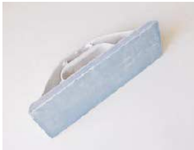
Figure 2. A rubber trowel is essential for grout work, because it forces grout into joints without marring the tile surface.
