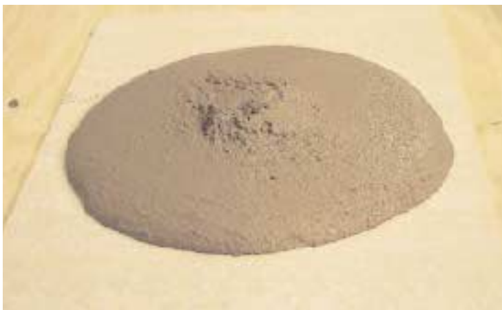
Figure 5. The consistency of the grout mix should be stiff enough to hold its shape, but fluid enough to fill joints when pressed into place with a rubber trowel. Mix subsequent batches in a clean bucket to keep the old grout from causing the fresh batch to set up too fast.
