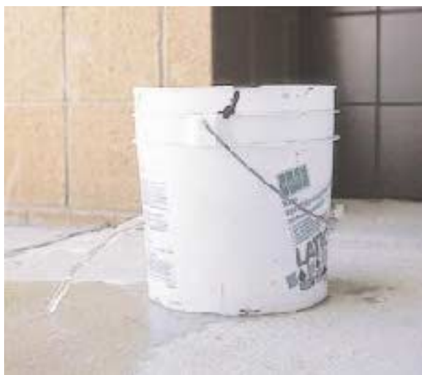
Figure 4. To ensure a precise liquid-to-powder ratio, the author recommends using a balance-beam scale for dry powder and large-scale measuring cups for the liquid. For larger quantities, he uses an “idiot bucket” — a plastic pail with a hole drilled in the side through which excess water can drain.
